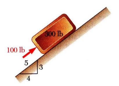
A 100 lb force acts as shown on a 300 lb block placed on an inclined plane. The coefficients of friction between the block and plane are  $\mu_s = 0.25$  and  $\mu_k = 0.20$ . Determine whether the block is in equilibrium and find the value of the friction force.
